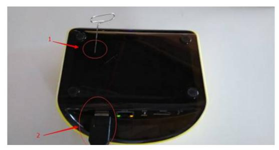
Press the reset key on the box then plug on the power. wait about 15sec,unloosen the reset button. and it will enter the recovery interface.
